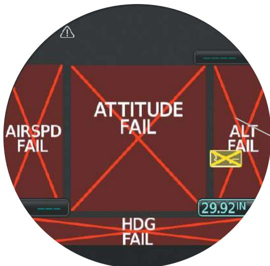
Red or Yellow 'X' Annunciation Indicates System Component Failure
