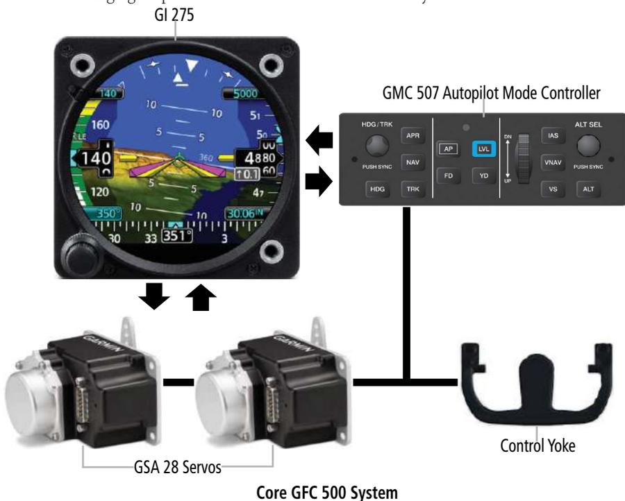
In addition to the core autopilot functions, the GFC 500 incorporates an independent monitor that uses inertial sensors to determine what is happening to the aircraft. By monitoring aircraft attitude, attitude rate and accelerations using these independent sensors, the monitor can shut down the autopilot if it determines the aircraft has exceeded predetermined limits.
