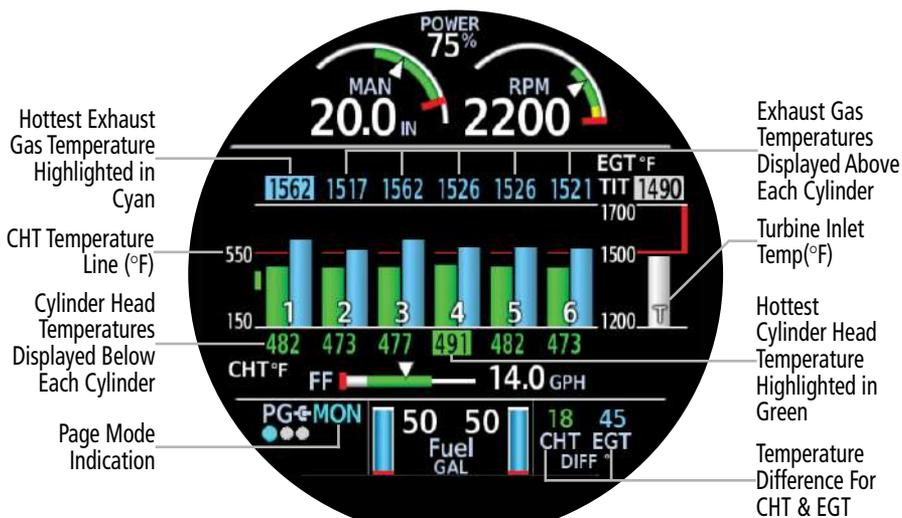
CHT/EGT - Six Cylinders - Turbine Inlet Temp
